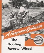
Side draft is effectively controlled in the Ferguson Disc Plow by means of the exclusive Ferguson Floating Furrow Wheel. Tilted-axle mounting keeps the furrow wheel of the Ferguson Disc Plow constantly operating at a transverse angle to the furrow wall . . . regardless of depth or width of plowing . . . completely absorbing all side-thrust of the plow.
